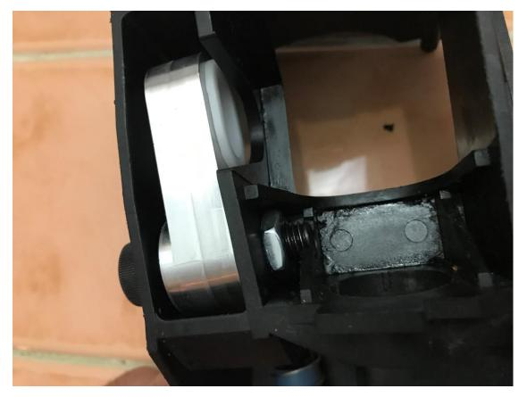
6. Now, remove your cable end (blue one) from the old lever. It's just a friction fit plastic pin.
