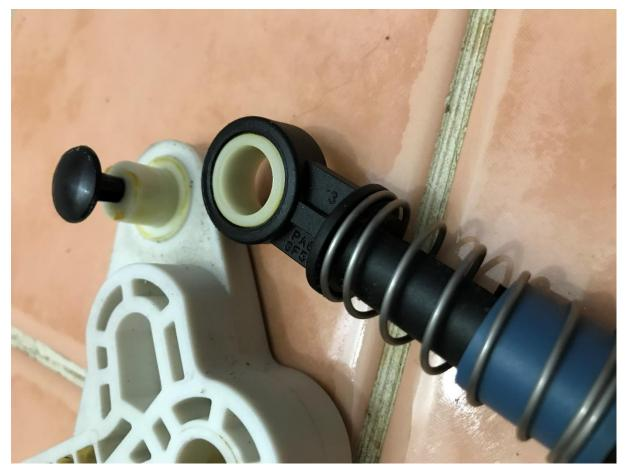
Grease it (any mechanical grease will do), and insert the new shaft with bolt on the aluminum lever. The use of thread locker is recommended here.
