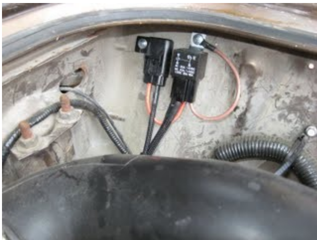
Suggested mounting location for hard start relay.
